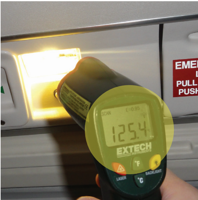
LED temperature indication under full power, about 125 deg F.
