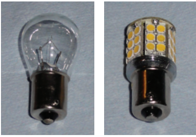
Baggage compartment bulbs, note the 307 is on the left and the 45 SMD BA15S LED bulb is on the right.
