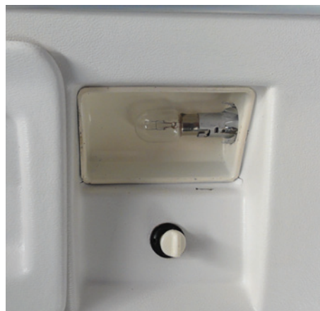
Passenger reading light in overhead cabin panel with lens removed, CM1495 incandescent bulb installed.
