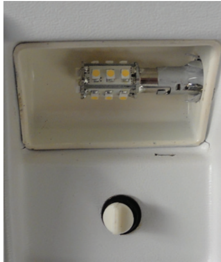
SMD Mini-tower LED bulb installed in passenger reading light fixture.
