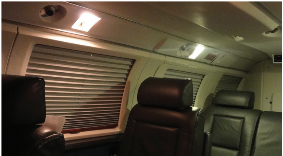
Passenger cabin illuminated with incandescent forward, and LED in the back. The light is just as bright and slightly less yellow.
